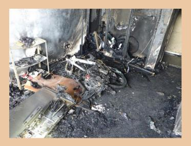
Lithium-ion batteries used to power new transport can cause ferocious and explosive fires if they are of poor quality or are mis-used.
