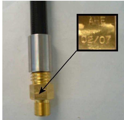
Figure 4.3: Aeroflex hose identification – Hard stamped
