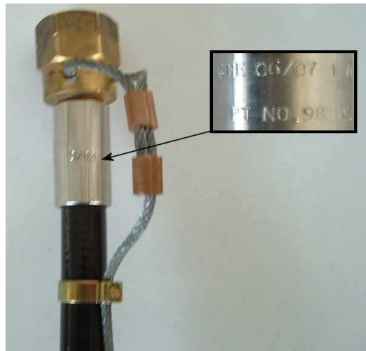
Figure 4.4: Aeroflex hose identification – Roll marked or etched
